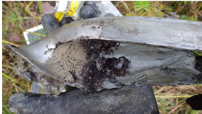
Figure 3.211: A soil core revealing a soil that was buried by a landslide in Lyman, Maine. The darkest layer in the middle of the core was the topsoil and the grey layer on the right was the bottom of the landslide (in this case, consisting of Presumpscot Formation). Plant fragments from the buried soil layer were sent for radiocarbon analysis to estimate the landslide age. Photo: Maine Geological Survey
